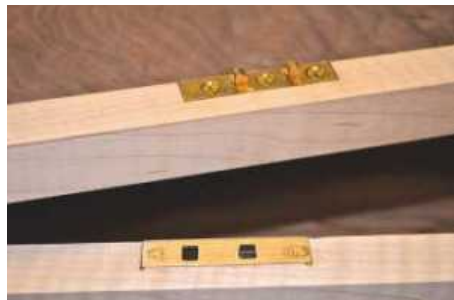
▲ Pic.17 For the lid part of the lock, where the upper plate goes that the lock grabs, I put the upper plate in the lock and locked it. That left the flat part of the plate pointing up. Then marking that piece with chalk, I set the lid back down on the plate and gave it a tap. After raising the lid, the chalk mark showed exactly where I had to cut out the lid portion for the upper plate to be inserted. Using a 3mm straight-fluted bit, I carefully routed out the hole for the upper plate, again chiselling out the inside corners, ensuring the plate sat flat and flush in the lid. After test fitting the locked box lid, I screwed in the upper plate. A word of caution: brass screws are soft; the heads can easily twist off in hardwoods if the hole is too tight. Always pre-drill your holes and use a steel screw of the same size to check for fit. Remove the steel screw and scrape a little candle wax on the brass screw threads before tightening down
